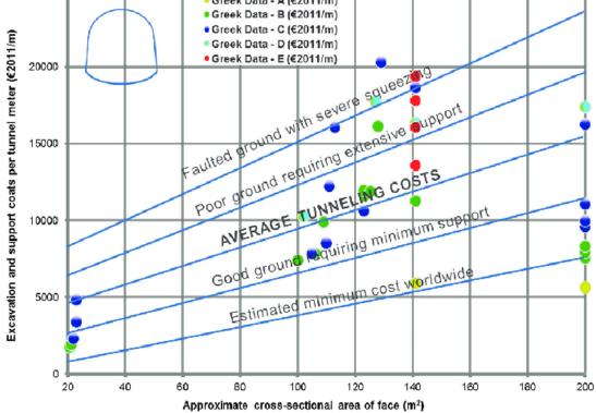
Tunnelling differs from the construction of other infrastructure in a plethora of ways. The main issues that distinguish tunnels from other infrastructure arise from the risk involved with excavation through unknown ground conditions and the numerous individual cost drivers that contribute to the overall cost. These cost drivers include, but are not limited to the following direct and indirect factors, all of which must be accounted for in our analysis.
