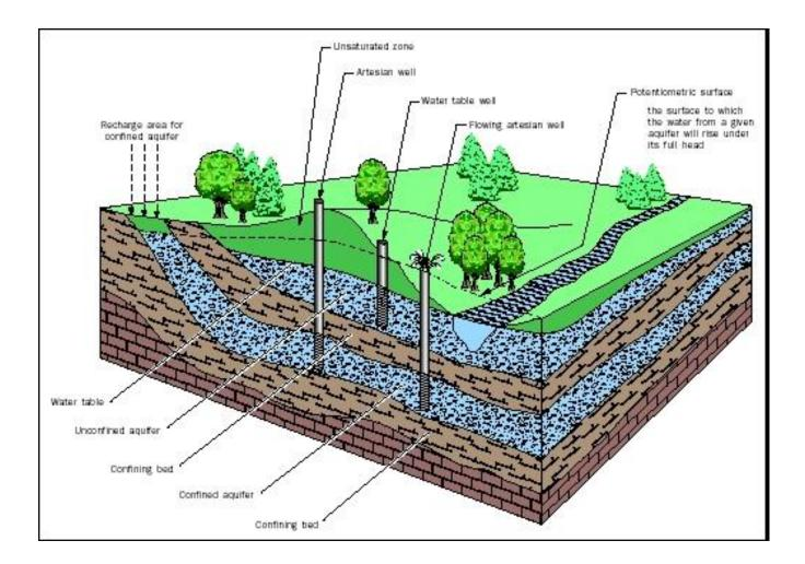
Water in a sand aquifer tends stay in place or move very slowly. Water injected into unconfined sand forms a stationary dome, and if there are confining layers then water spreads out horizontally.
