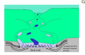
**Figure 2** – Intact valley floodplain. Discontinuous low velocity flow. Retention and recycling of water and nutrients. Freshwater lens over saline groundwater. Note that main flow path is on the highest part of the floodplain At the same time, hydrostatic pressure from the perched water table in the stream prevents the lateral intrusion of salinity from the floodplain even in low flow periods.
