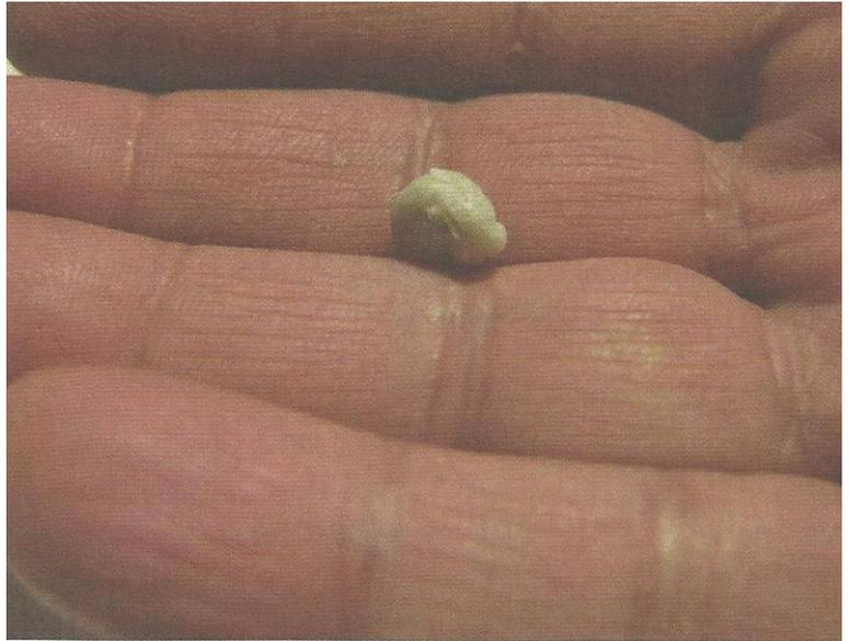
Fig. 30 D: Solid CO<sub>2</sub> material in the gas-state held at room temperature. This solid CO<sub>2</sub> is not 'dry ice' but a mastic-like matter.
