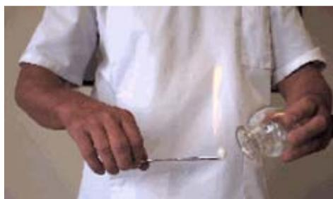
*Using a burning cotton wool ball to create a vacuum inside a glass cup*
