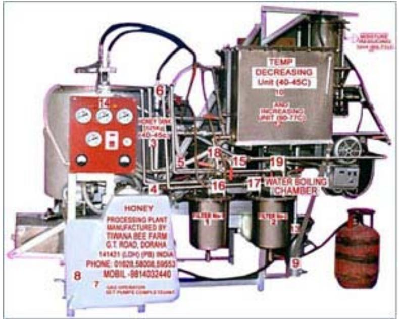
Tiwana Honey Processing Plant ensures processing of raw honey hygienically to meet best possible quality standards. All the parts that come in contact of honey are made of stainless steel to ensure high product quality and hygiene. Electricity requirement for the entire plant is just 2 KW. Thus it is well in reach of a small innovative entrepreneur to produce high quality honey.
