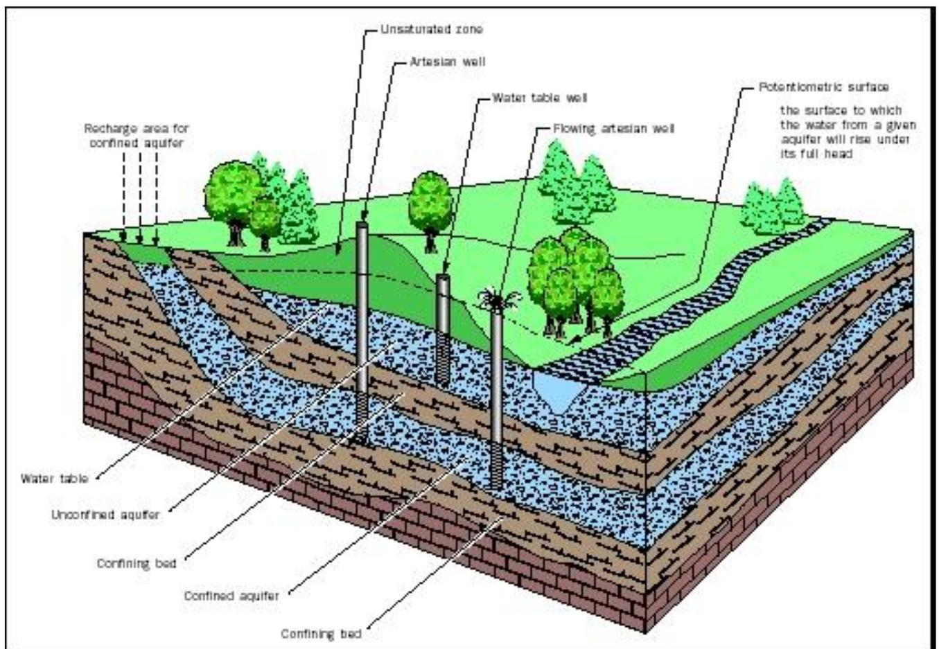
Water in a sand aquifer tends to stay in place or move very slowly. Water injected into unconfined sand forms a stationary dome, and if there are confining layers then water spreads out horizontally.
