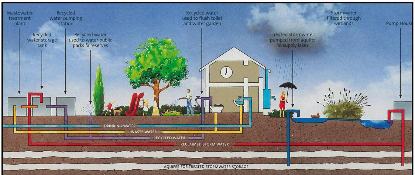
Aquifer Storage and Recovery (ASR) is the process of injecting water into a suitable underground aquifer for storage and later reuse, and it can be a means of artificially recharging depleted underground water supplies.
