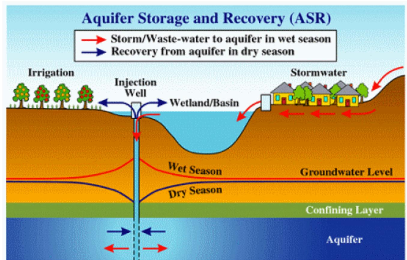
Aquifer Storage and Recovery (ASR) involves injecting water into an aquifer through wells or by surface spreading and infiltration and then pumping it out when needed. The aquifer essentially functions as a water bank. Deposits are made in times of surplus, typically during the rainy season, and withdrawals occur when available water falls short of demand.
