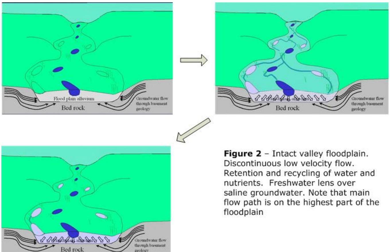
**Figure 2** – Intact valley floodplain. Discontinuous low velocity flow. Retention and recycling of water and nutrients. Freshwater lens over saline groundwater. Note that main flow path is on the highest part of the floodplain
