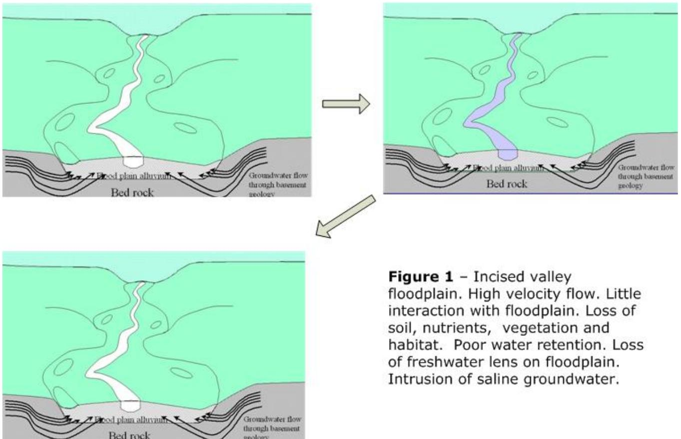
**Figure 1** – Incised valley floodplain. High velocity flow. Little interaction with floodplain. Loss of soil, nutrients, vegetation and habitat. Poor water retention. Loss of freshwater lens on floodplain. Intrusion of saline groundwater.
